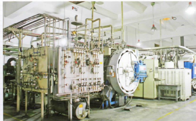
压力烧结炉能极大地改善合金的组织结构 Sinter HIP-can improve the microstructure of the cemented carbide by eliminating the porosity
