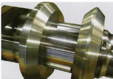
型钢轧制用硬质合金复合轧辊 Combine roll for profile mill
