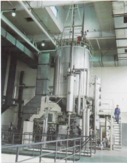
喷雾干燥塔用于生产高品质原料 Spray dryer for manufacturing high quality materials
