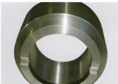
窄带钢轧制用复合辊环 Composite roll for strip steel rolling
