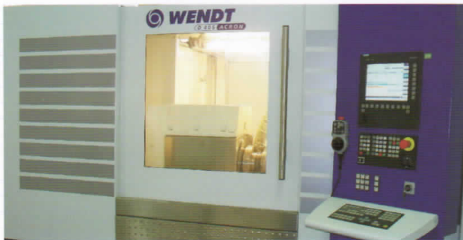
进口专用磨床用于高精度滚环的加工 Introduced special grinding machine for processing high precision roll-rings
