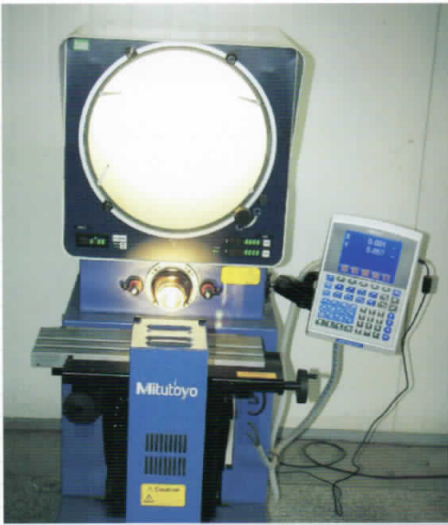
投影仪 Optics projection apparatus
