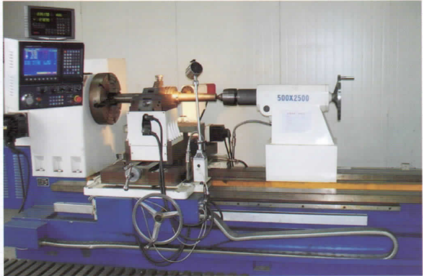
刻痕机用于螺纹滚环精密加工 Special machine for processing high precision thread roll-rings
