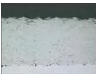
Cross-section metallograph of WC-10Ni coatings
