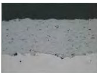
Cross-section metallograph of WC-15NiCr coatings
