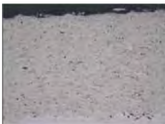
Cross-section metallograph of Cr 3 C 2 -37WC-18NiCoCr coatings
