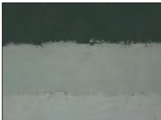
Cross-section metallograph of WC-17Co coatings
