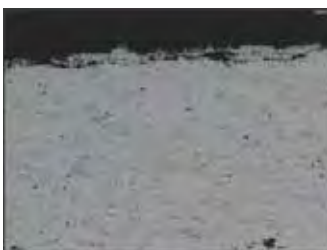
Cross-section metallograph of Cr 3 C 2 -25NiCr coatings
