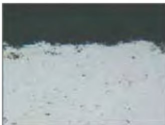
Cross-section metallograph of WC-12Ni coatings
