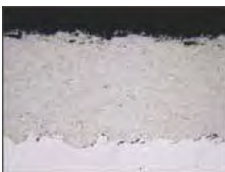
Cross-section metallograph WC-20Cr 3 C 2 -7Ni coatings
