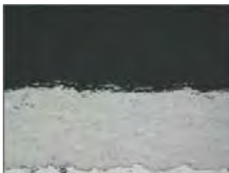
Cross-section metallograph of WC-9Co5Cr1Ni coatings
