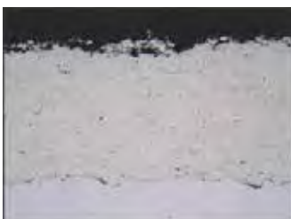
Cross-section metallograph of Cr 3 C 2 -20NiCr coatings
